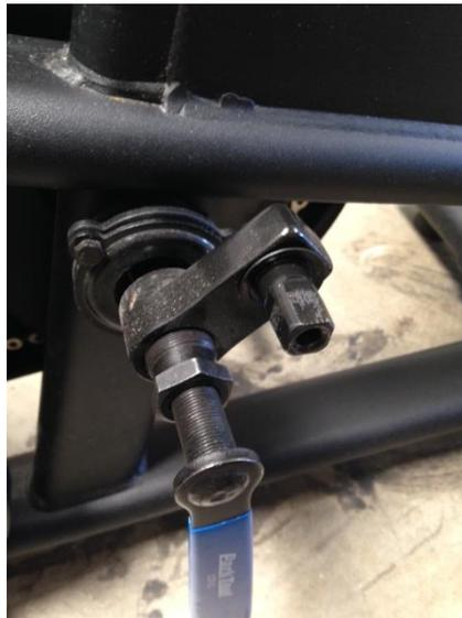
**Step 5:** After the Crank Fixing Bolt (part#42) is removed install the crank puller and then remove the Bell Crank (part#40).
