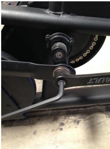
**Step 1:** Using the 8mm hex wrench rotate the Crank Fixing Bolt (part#42) counterclockwise to remove.
