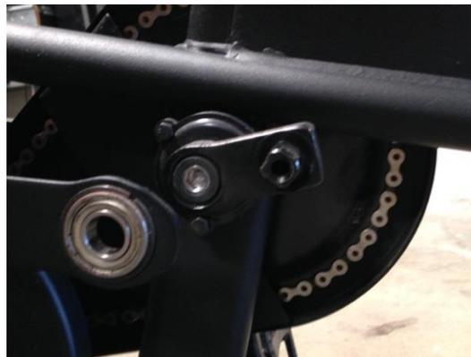
**Step 3:** After removing the crank arm remove the Linkage Arm (part#12) exposing the Bell Crank (part#40). When the Linkage Arm is removed also remove the thin plastic washers that are between the Linkage Arm and the Bell Crank. Your unit may or may not have the plastic washers.
