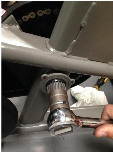
**Step 3:** After the Bottom Bracket Lock ring is removed install the Shimano/ISIS Bottom Bracket removal tool. Once the tool is installed rotate the Bottom Bracket shell **counter clockwise** until it comes off.
