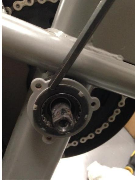
**Step 2:** Using the Allen wrench or the flat screwdriver tap the Bottom Bracket Lock ring counter clockwise.
