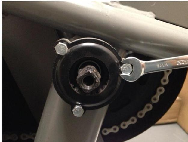
**Step 1:** Using the 8mm wrench remove the 3 Hex Screws (part#39). Once the screws are removed, remove the Bottom Bracket Locking Plate (part#38).
