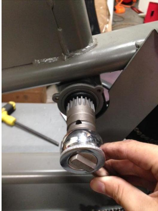
**Step 4:** On the right side of the machine install the Shimano/ISIS Bottom Bracket removal tool. Once the tool is installed rotate the Bottom Bracket shell **clockwise** to remove.
